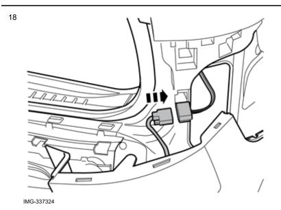
Place the Bumper Cover in position for installation.
