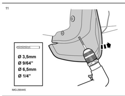
Bend the mudflap backwards and drill a 3.5 mm (9/64") hole in the marking underneath.
