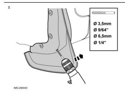
Bend the mudflap backwards and drill a 3.5 mm (9/64") hole in the marking underneath.
