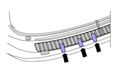
Adjust the position of the Bumper Protection using the tape marks.
