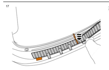
Allow the Bumper Protection to adhere to the Bumper Cover as indicated.
