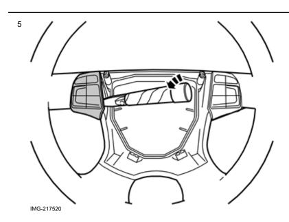
Remove the left keypad/keypad dummy from the steering wheel by carefully prying it off using a plastic weatherstrip tool. Twist the weatherstrip tool to pry it out. The keypad/keypad dummy is firmly held in place by three lugs in the steering wheel, so some force is required to remove it.
