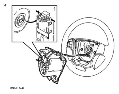
Insert a screwdriver in the hole (1) on the reverse of the steering wheel, at right angles to the rear surface of the steering wheel. Insert the screwdriver as far as possible to determine the position of the end of the spring clip (2).
