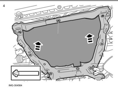
Remove the clips for the protective plate mounting in the subframe.
