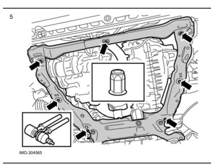
Take the rivet nuts from the kit and tighten in the drilled holes. Use tool  $\ensuremath{\mathsf{P/N}}$  9512782.
