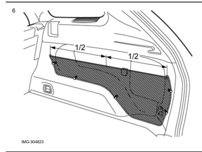
Measure out half the distance between the net pocket's eyelets and mark on the side panel, about the same height as the two eyelets.
