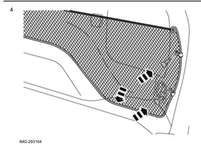
Take screws and the mesh from the kit. Tighten the screws at the rear edge of the mesh pocket, with the mesh pocket positioned towards the lower edge of the side panel.
