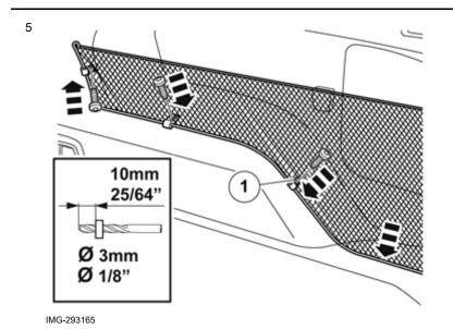
Fold the mesh pocket towards the side panel and ensure that it is against it at the arrow markings.
