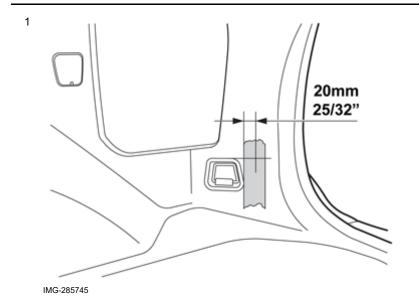
Attach a piece of tape edge-to-edge with the panel for the rear load securing eyelet as illustrated. Measure and mark out for drilling holes for the lower rear clip.
