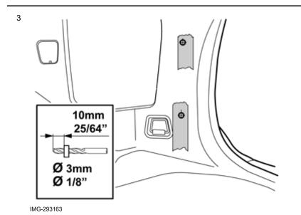
Drill two Ø3 mm (1/8") holes through the panel. Use a 10 mm (25/64") drill stop.
