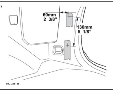
Attach a piece of tape on top of the previous one as illustrated. Measure for drilling the upper hole for the clip.
