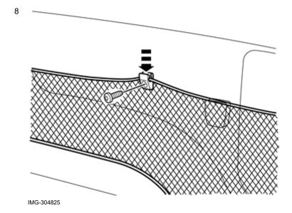
Get clips and screws from the kit and tighten down.
