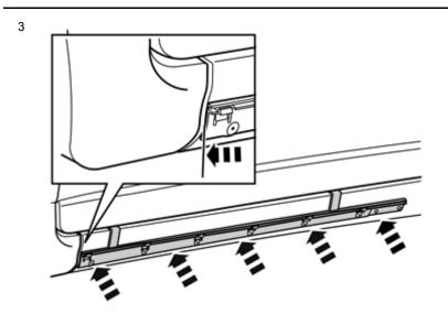
Align the front edge of the cradle with the rear edge of the joint between the sill panels. Ensure that the tape does not adhere yet. At the same time hook the cradle on the top of the sill panel.
