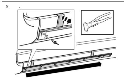
Rivet the cradle in all holes at the sill panel. Break off the hooks along the cradle.
