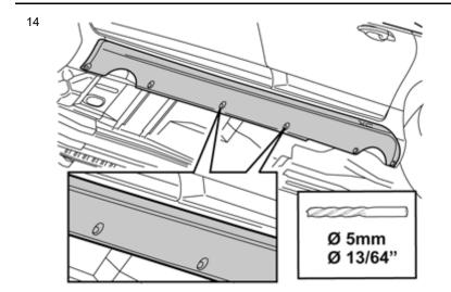
Press the lower part of the panel towards the sill panel at the middle holes and drill through both using a Ø 5 mm (13/64") drill bit.
