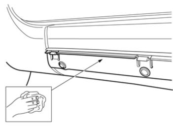
Rivet the cradle in all holes at the sill panel. Break off the hooks along the cradle.
