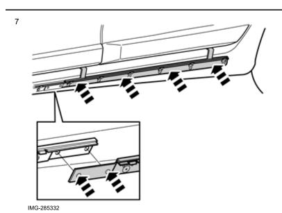
Align the lugs on the cradle with corresponding holes in the front cradle. Ensure that the tape does not adhere yet.
