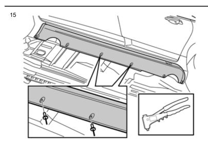
Rivet the panel through the two holes.
