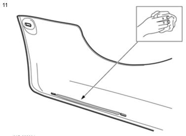
Clean the marked area on the protrusion between both mounting hooks on the front edge of the decor strip using isopropanol and wipe dry.
