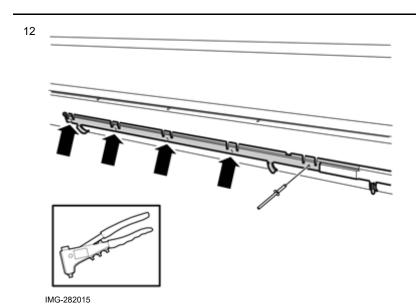
Take pop rivets from the kit. Rivet the holder to the door sill panel.
