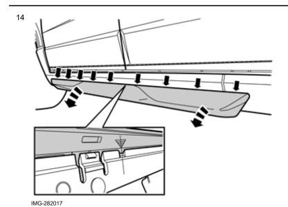
Hook the sill decor onto the holders. Start opposite the marking on the decor strip and cut-out, at the rear section of the front holder
