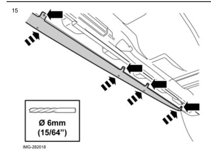
Press in the sill decor opposite the mounting eyelets against the underneath of the door sill panel. Drill out the holes through these using a  $\emptyset$ 6 mm (15/64") drill bit. Remove any swarf.
