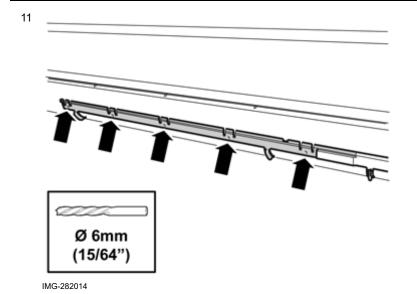
Drill out the five marked holes in the holder using a  $\emptyset 6$  mm (15/64") drill bit.
