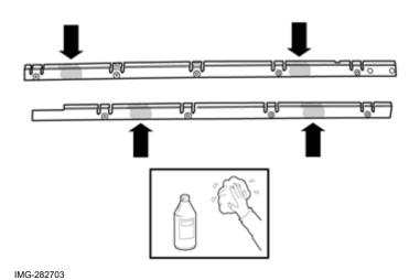
Take a rear and front holder from the kit. Clean the surfaces that are to be positioned against the door sill panel where the pieces of tape are to be positioned. Use isopropanol.
