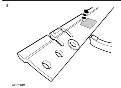
Remove the protective tape from the mounting tape on the front holder.
