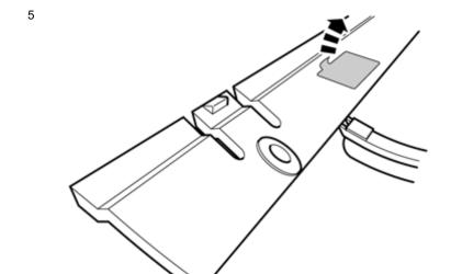
The holders are marked and only fit in one place. Start with the rear holder.
