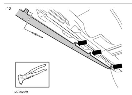
Rivet the mounting eyelets to the body using pop rivets.
