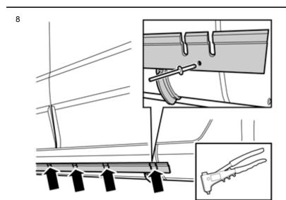
Take pop rivets from the kit. Rivet the holder to the door sill panel.
