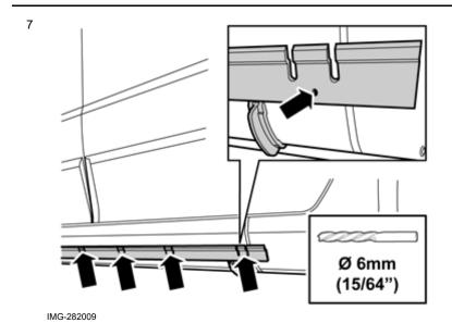
Drill out the four marked holes in the holder using a  $\emptyset$ 6 mm (15/64") drill bit.
