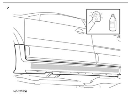
Clean the door sill panels using isopropanol where the decor panel's holder is to be positioned.
