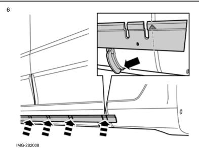
Align the ends of the markings that are at the rear edge on the rear holder, with the front part of the joint between the door sill panels.
