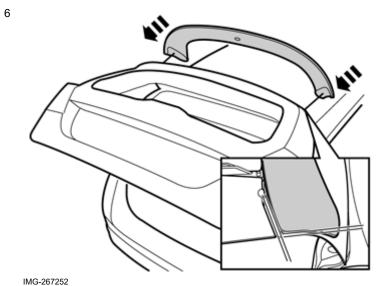
Do not remove the protective tape from the spoiler yet.
