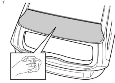
Wash the outside of the upper section of the boot lid and wipe dry.
