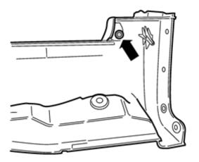
Detach the door sill panel's front end. It is secured by a clip.
