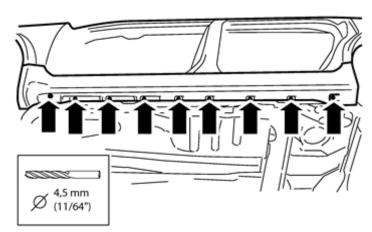
Drill out the central pins in the clips at the lower edge of the door sill panel and remove them. Use a Ø4.5 mm (11/64")
