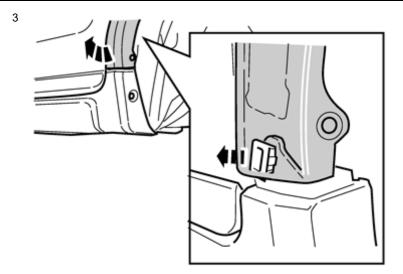
Carefully turn out the lower edge/rear edge of the front end of the wing extender.
