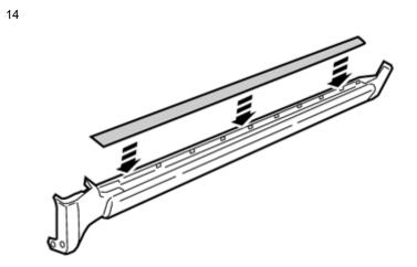
Press the rubber strip onto the new panel.
