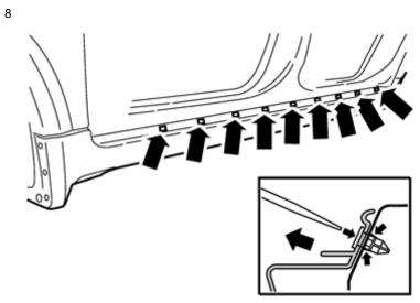
Insert a large flat-bladed screwdriver, press the bottom of the clips and pull off the door sill panel with the clips.
