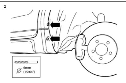
Drill out the pop rivet at the rear edge of the door sill panel and the rear pop rivet in the wing extender. Use a Ø6 mm (15/64") drill bit.
