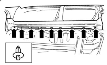
Press the panel into place in the lower edge using new clips.
