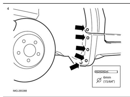
Drill out the pop rivets at the front edge of the door sill panel and in the rear edge of the wing extender. Use a Ø6 mm (15/64") drill bit.
