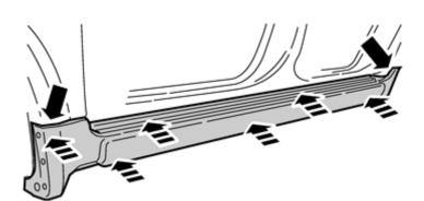
Align the door sill panel ends under the wing extenders.
