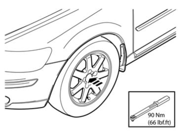
Install the front wheel. Tighten to the correct torque.
