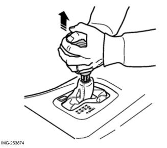
Pull loose the gear lever knob by forcefully pulling it straight upward.
