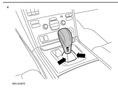
Check that the gaiter's seams are straight. Then fix the lock ring by pulling it down and the gaiter straight up against the knob, and secure it by pressing it into place.
