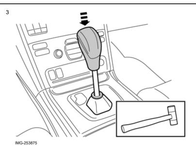
Place the new knob in the correct position on the gear lever.
