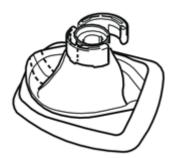
Turn the gear selector lever gaiter inside out.
