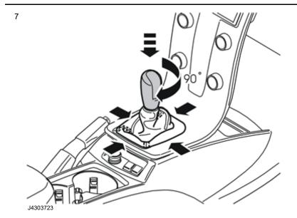
Turn the inside of the gear selector lever gaiter back in.
