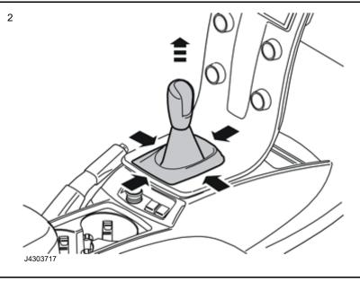
Remove the gear selector lever knob with gaiter by prizing loose the gaiter from the centre console at the catches where indicated by the arrows, and then pull the whole unit up.
