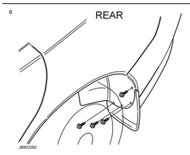
Clean around the screw holes in the rear edge of the wing liner
