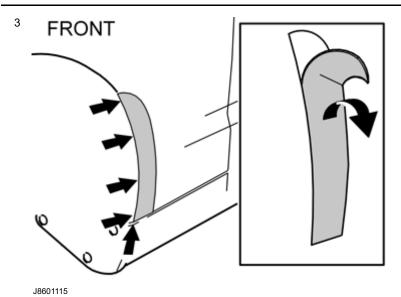
Remove the backing from the masking tape
