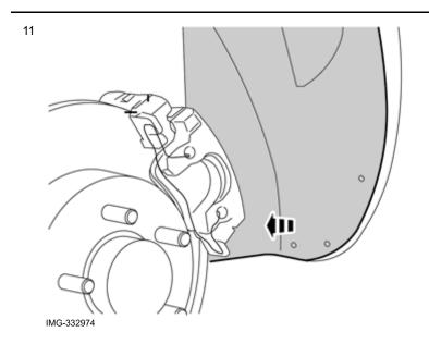
Fold the wing liner out of the way.
