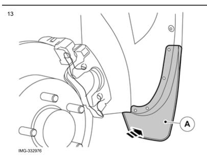
Fold the inner wing back and install the mudflap.
