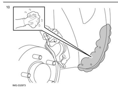
Clean the area where the mudflap is to be positioned.
