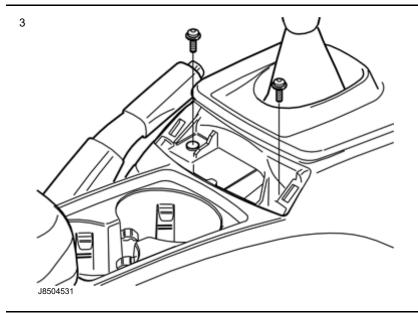
Remove the two screws holding the centre console at the rear edge.
