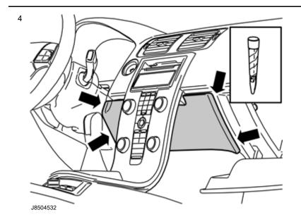
Remove the panel on the rear of the centre console:
