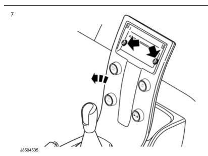
Remove the two screws holding the centre console to the dashboard.
