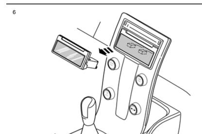
Press out the display module from the reverse of the centre console. Press straight backwards, using both hands.
