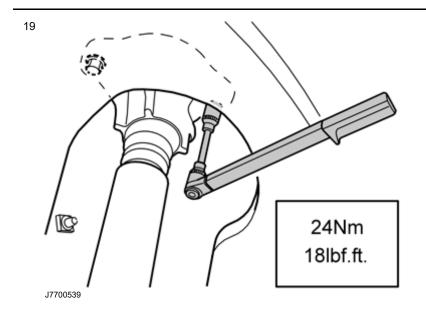
Tighten the shock absorber upper bearing to the body and tighten the screws to 24 Nm (18 lbf.ft).
