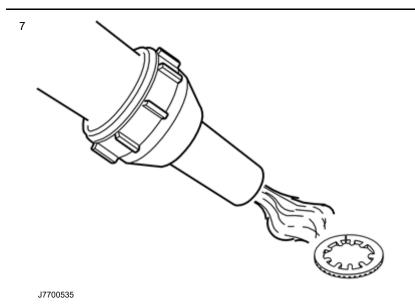
Take the hot air gun and warm up the spacer washer so that it can be eased over the steering gear rack.
