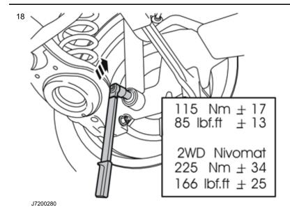
Reinstall the shock absorber in its lower mounting and tighten the screw to 115 Nm  $\pm$  17 (85 lbf.ft  $\pm$  13). For 2WD Nivomat, the torque on the screw must be 225 Nm  $\pm$  34 (166 lbf.ft  $\pm$  25).
