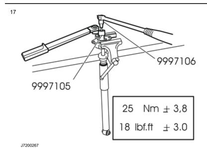
Reinstall the upper bearing for the shock absorber and tighten the nut to 25 Nm  $\pm$  3.8 (18 lbf.ft  $\pm$  3.0).
