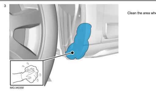
Clean the area where the mudflap is to be positioned.
