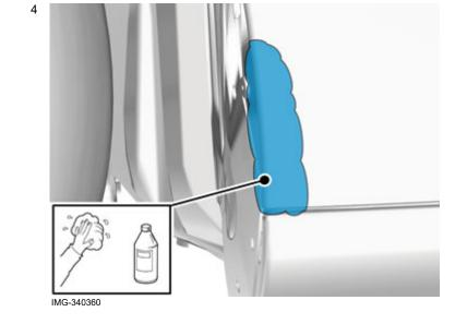
Clean the area where the protective tape is to be attached. Use: Isopropanol.
