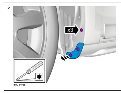
Remove the screws and flap. These will not be reused.
