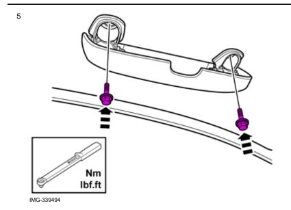
Torque tighten the screws to 8Nm (6 lbf.ft.)
