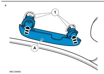
Make sure that the four retaining plates (1) sit on each side of the nut plates where the glasses holder will be fastened. If there is not enough room for the plate, it can be broken off and discarded.
