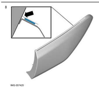
**Note!**Apply protective foil edge to edge with the part.
