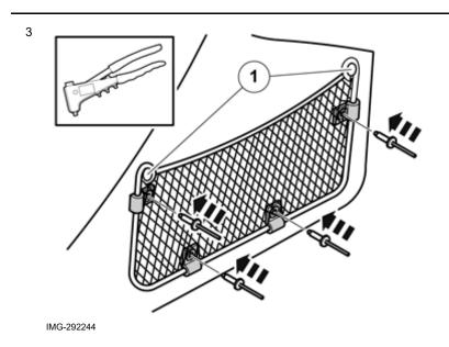
Position the mesh pocket with the clips against the holes in the side panel. Turn the pocket's buttons (1) outwards.
