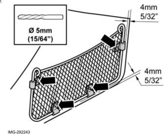
Place the mesh pocket on the panel with the front edge of the clips 4 mm (5/32") from the panel's front and rear edge. Attach the mesh pocket using tape to secure it.
