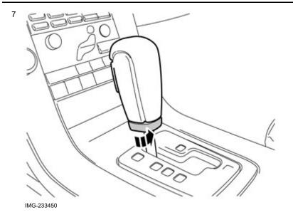
Turn the locking sleeve on the gear selector lever knob a quarter turn counter-clockwise.
