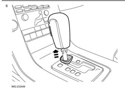
Move the locking sleeve up over the catches.
