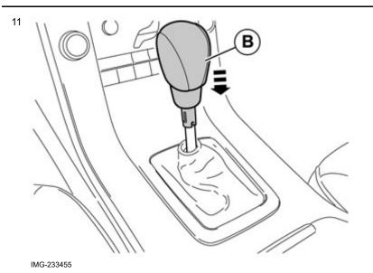
Install the new gear selector lever knob.
