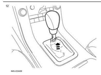
Move the boot and locking ring up so that the locking ring hooks into the gear selector lever knob.
