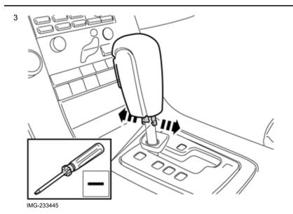
Pry out the 2 x catches at the front and rear edge using a small screwdriver.
