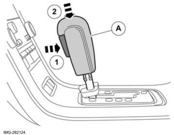
Install the new gear shift knob (A) by first pressing in the lock button (1). Then push it down (2) until the catches engage.
