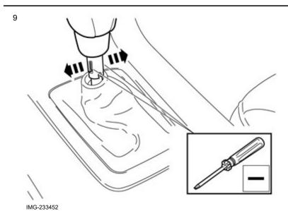
Pry out the 2 x catches on the side using a small screwdriver.
