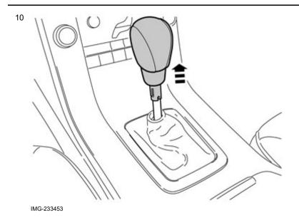
Pull the gear selector lever knob straight up.
