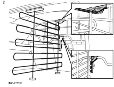
Position the cargo compartment wall with the clamps into the car.
