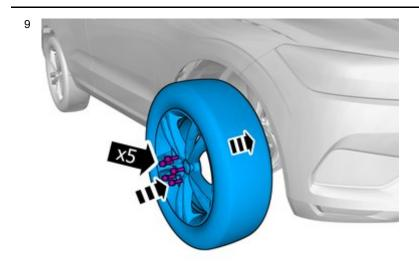
**Tightening torque:** Wheel to wheel hub Stage 1: 20 Nm Stage 2: 140 Nm
