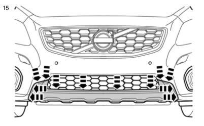
Now press the skid plate into place opposite the tape all the way around.
