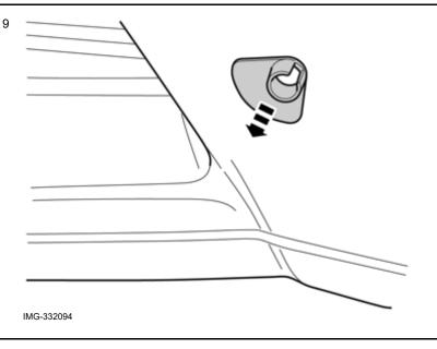
Remove the drilling templates on both sides.
