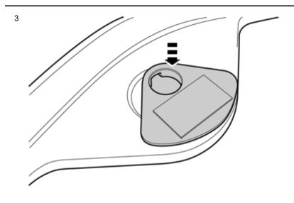
Take the drilling template and skid plate from the kit and press the drilling template into the hole in the mounting lug to the clip's mounting.
