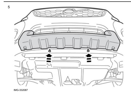
Secure the skid plate using existing screws. Do not tighten excessively so that the position can be adjusted laterally. Ensure that the tape on the drilling template does not adhere yet.
