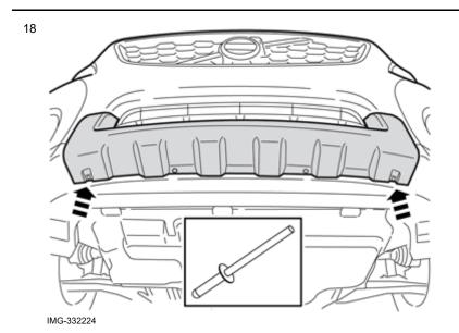
Take the rivets from the kit and rivet the skid plate in the outer ends.
