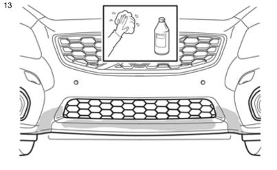
Clean the marked surfaces for the tape to the skid plate using isopropanol.
