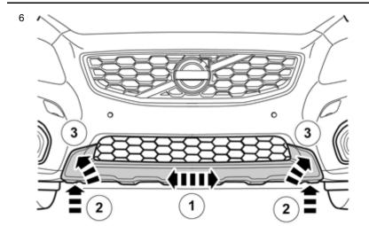
Now position the skid plate laterally (1). Ensure that the tape on the drilling templates does not adhere yet.
