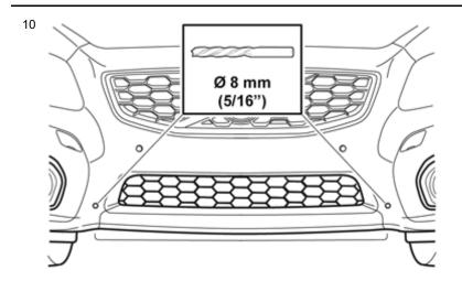
Drill the holes to Ø 8 mm (5/16 ").
