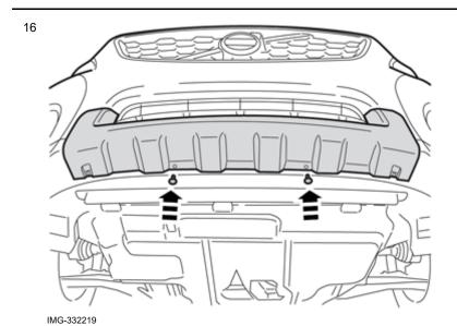
Tighten the skid plate underneath using existing screws.
