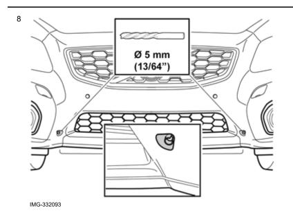
Drill out the holes through the taped drilling templates.
