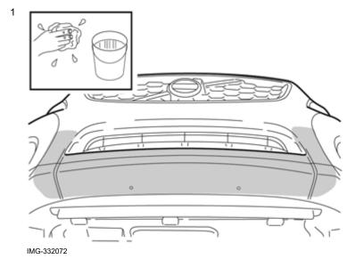
Wash the surfaces of the car that are to be covered by the skid plate.
