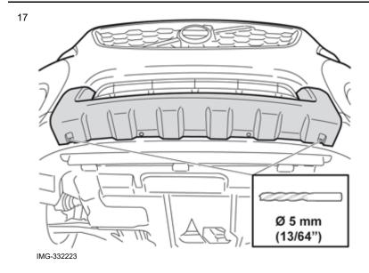
Drill through the existing holes in the outer ends of the skid plate and through the air baffle.
