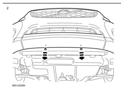
Remove the two centre screws from the air baffle. They will not be reused.
