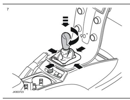
Turn the inside of the gear selector lever gaiter back in.
