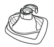
Turn the gear selector lever gaiter inside out.
