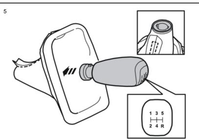
Guide the gear selector lever knob inside the out-turned gear selector lever gaiter. The text on the gear selector lever knob must point from the seam in the gaiter.
