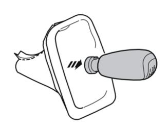
Pull the gear selector lever knob away from the gaiter.
