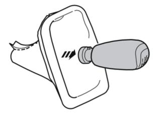
Pull the gear selector lever knob away from the gaiter.
