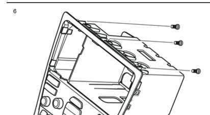
Remove the three screws in the upper edge of the trim for the unit and radio and dashboard environment panel.
