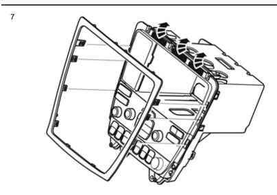
Remove the trim from the unit. Pry off the catches along the vertical and lower sides of the trim. Pull off the trim. Do not damage the catches. The catches are thin and easily broken
