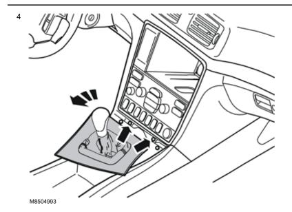
Apply the handbrake. Move the gear selector backwards
