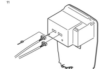
Reconnect the connector for the phone, if installed
