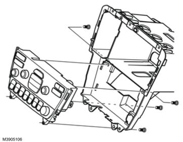
Remove the four screws on the reverse of the dashboard environment panel. Remove the dashboard environment panel from the bracket.
