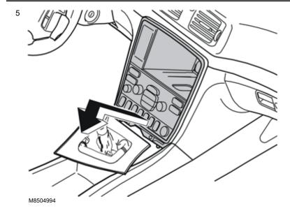
Remove the bracket with dashboard environment panel from the centre console: Pull the lower edge out and downwards until it releases from the mounting at the upper edge. Then fold backwards.
