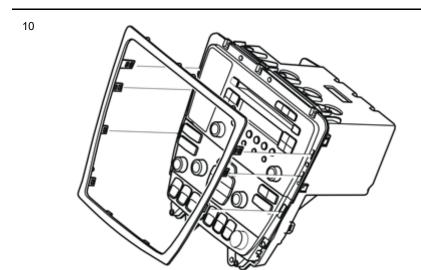
Reinstall the dashboard environment panel in the bracket. Use 4 x screws
