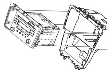
Take the radio from the kit. Press the radio into place in the bracket. Ensure that all the four catches on the sides engage.
