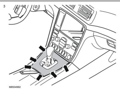
Detach the rear edge of the gear selector lever cover together with the boot until the two clips release. Use a plastic weatherstrip tool. Remove the gear selector lever cover and the boot. Pull the panel up until the four clips at the sides release.
