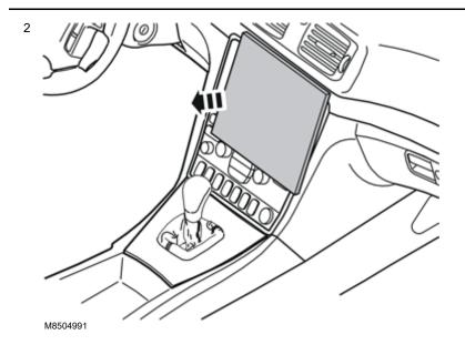
Remove the polystyrene block from the centre console. It will not be reused.
