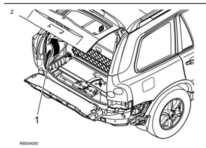
Remove the left-hand side floor hatch (1).
