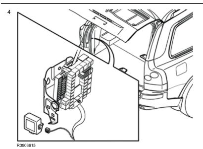
Disconnect the pre-routed green connector, taped on the cable harness under the fuse holder
