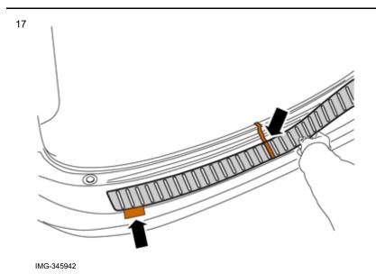
Adjust the position of the Bumper Protection using the tape
