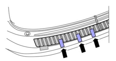
**Note!**Use tape to temporarily fix the bumper cover in the correct position.
