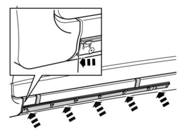
Align the front edge of the cradle with the rear edge of the joint between the sill panels. Ensure that the tape does not adhere yet. At the same time hook the cradle on the top of the sill panel.
