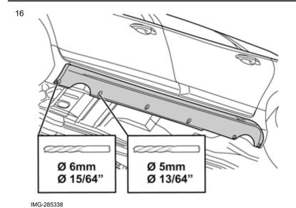
Press the lower part of the panel towards the sill panel at the front holes.
