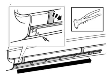
Rivet the cradle in all holes at the sill panel.
