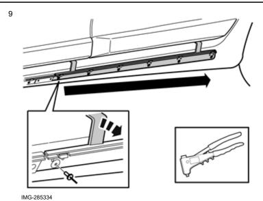
Rivet the cradle in all holes at the sill panel.
