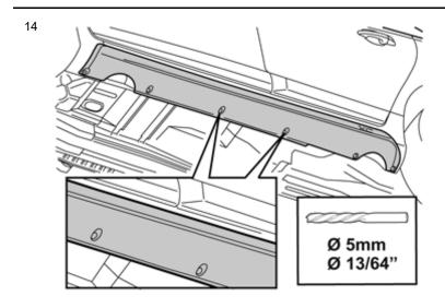
Press the lower part of the panel towards the sill panel at the middle holes and drill through both using a  $\varnothing$  5 mm (13/64") drill bit
