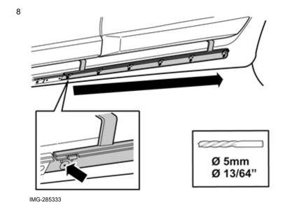
Drill out the six marked holes using a Ø 5 mm (13/64") drill bit.
