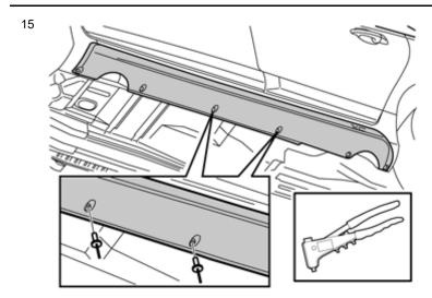
Rivet the panel through the two holes.
