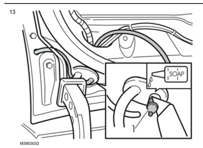
Cut the rubber nipple (1) off the rubber grommet for the brake lamp. Do not damage the existing cables
