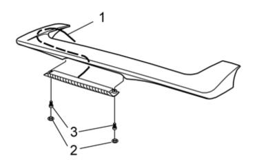
Route the cable (1) through the spoiler. Thread a piece of steel wire or a thin plastic rod into the hole for the cable lead-in starting at the brake lamp. Tape the terminal pins and cable to the steel wire. Pull out through the hole.
