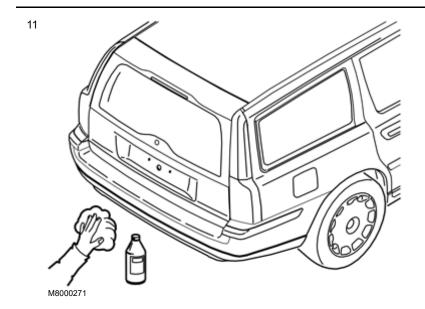
Clean the surfaces where the roof spoiler is to be installed. Use a mixture of 30% windscreen washer fluid and 70% water
