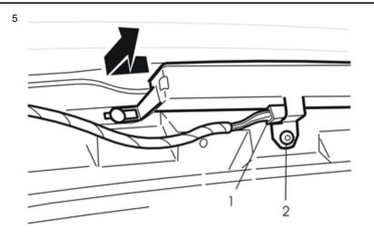
Remove the connector (1) from the brake lamp
