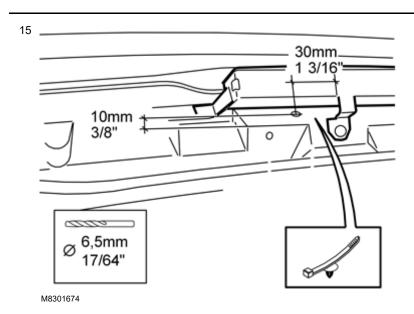
Drill holes in the tailgate for the attachment of the connector
