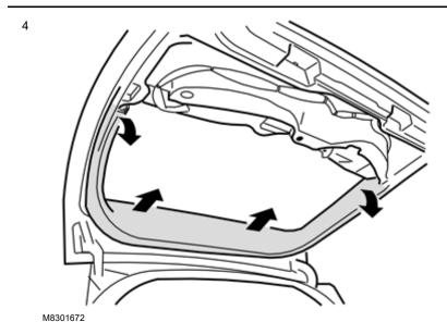
Pull down the sides of the panel around the tailgate window to release it from the two clips
