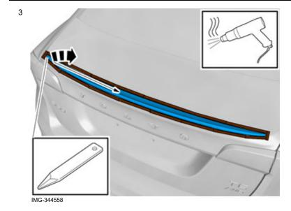
Heat around the edges of the spoiler and carefully pry it off using a weatherstrip tool. Do not damage painted surfaces.
