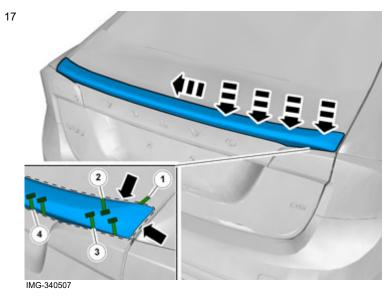
Carefully pull off the spoiler's protective tape, maintaining the position of the spoiler. Start by pulling off the protective tape (1) on the ends first, then at the front edge (2), then the short rear (3) then the long rear (4).
