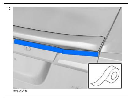
Remove the spoiler and tape along the marking on the boot lid's rear edge to prevent primer spillage. Fold up the lower edge of the tape so that any excess primer ends up there.
