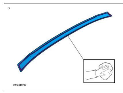
Wipe clean the protective tape on the spolier's attachment tape before marking up on the boot lid.
