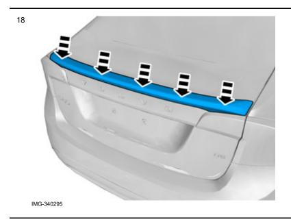
Press the spoiler so that the tape adheres properly. Clean off the markings using isopropanol.
