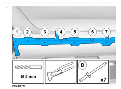
Drill one hole and fit one pop rivet at a time, in accordance with the sequence illustrated.
