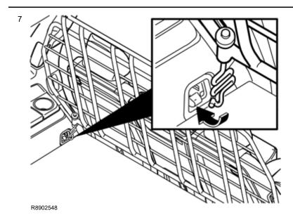
Insert the mounting bracket from underneath through the lower mounting in the cargo compartment safety grille as illustrated. Screw on the knob
