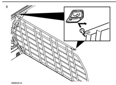
Lift the cargo compartment safety grille in through the tailgate or through one of the rear doors (fold down the second row of seats if using one of the rear doors)
