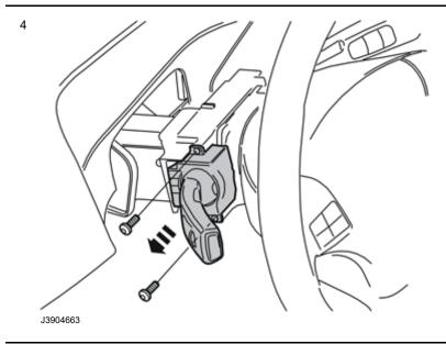
Remove the left-hand control stalk. First remove the two screws. Then carefully pull the stalk outwards until it releases from the connector on the inside.
