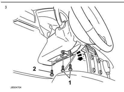
Remove the upper screws (1) from the lower steering column cover
