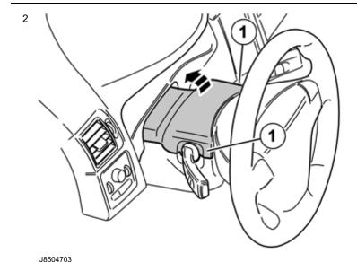
Carefully pry the upper steering column cover off the lower cover. Using a plastic weatherstrip tool, pry at the rear edge in the join between the steering column covers. The steering column covers are secured to each other by catches (1) on the inside
