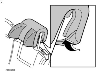
Pull the padded upholstery over the rear side of the head restraint and secure it around the rear lower edge of the head restraint.
