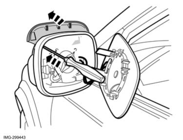
Press out the mirror's cover using a small screwdriver.
