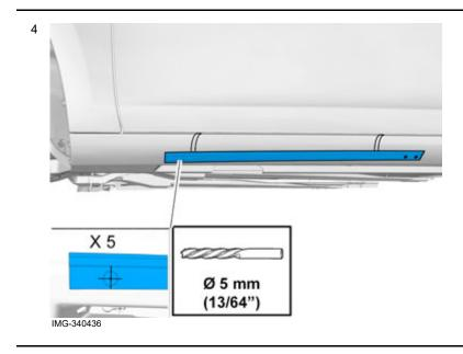
Drill out the five marked holes in the cradle using a Ø 5 mm (13/64") drill bit.
