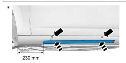
Align the front edge of the cradle according to the dimension measured from the front edge of the sill panel. Ensure that the tape does not adhere yet. Hook the cradle on the top of the sill panel.
