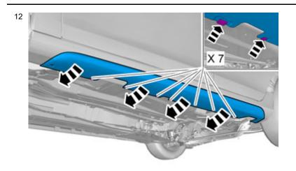
Take seven clips from the kit and secure the plate's lower edge at the lower edge of the sill panel at the pre-marked locations. Start with the two inner clips and continue out towards the ends of the panel.
