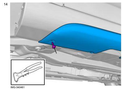
Take pop rivets and rivet the plate's front end.
