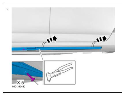
Rivet the cradle in all holes at the sill panel. Break off the hooks along the cradle.
