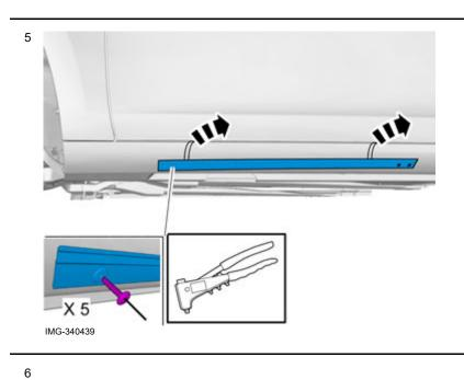
Rivet the cradle in all holes at the sill panel. Break off the hooks along the cradle.
