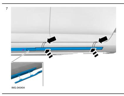
Align the lugs on the cradle with corresponding holes in the front cradle. Ensure that the tape does not adhere yet.
