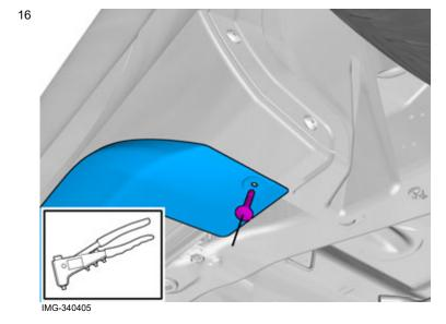
Take pop rivets and rivet the plate's rear end. Repeat the above for the other side.
