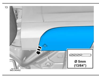
Fold the front edge of the plate around the lower edge on the sill panel properly and drill out the hole in the sill panel using a 5 mm (13/64") drill bit.
