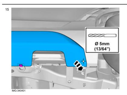
Fold the rear edge of the plate around the lower edge on the sill panel properly and drill out the hole in the sill panel using a 5 mm (13/64") drill bit.
