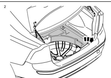
Remove the upper floor supports on the left and right-hand sides if applicable.
