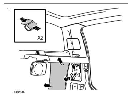
Remove the insulation panel on the right-hand side. The insulation panel is secured by two clips behind the rear wheel arch
