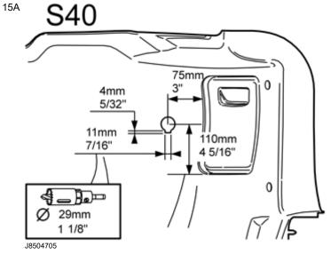
Applies to cars without marking for 12V socket. Image A applies to the S40 (04-)
