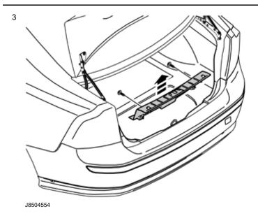
Unscrew the two external clips at the front edge/bottom edge of the sill trim panel on the tailgate.
