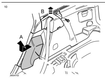
Grasp the upper edge of the right-hand side cushion. Pull the side cushion forward so that the clip on the reverse releases (A).
