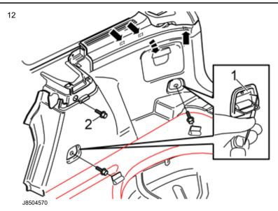
Fold out the load securing eyelets on the right-hand side panel.
