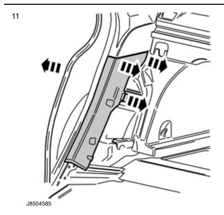
Pull off the rubber strip at the rear of the opening for the right-hand rear door.
