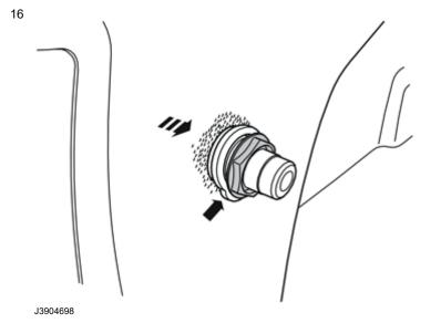
Install the 12V socket in the hole in the panel. Install the space washer and nut, and tighten.
