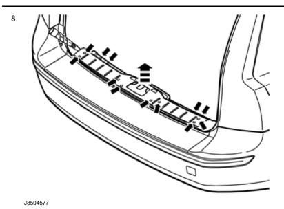
Prize off the four external clips at the front edge/bottom edge of the sill trim panel on the tailgate.
