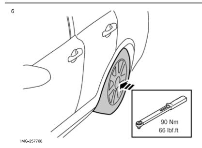
Reinstall the rear wheel, tightening torque 90 Nm (66 lbf.ft).
