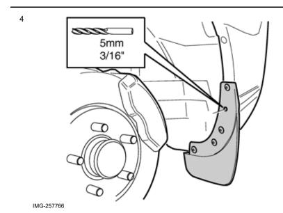
Drill a Ø5 mm (3/16") hole for the pop rivet.
