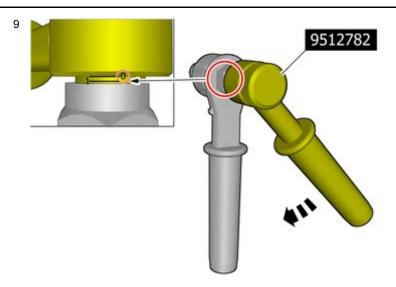
Use special tool: T9512782, Rivet nut tool
