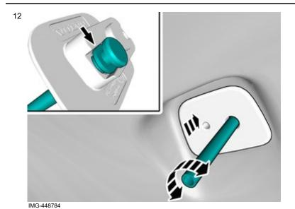
Turn marked detail while pushing the mounting to make the detail fit the mounting outlet
