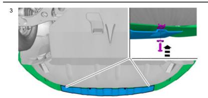
Tighten the skid plate at the outer ends.
