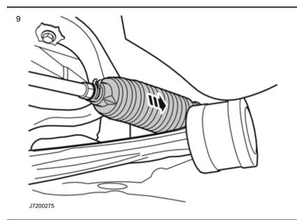
Reinstall the rubber gaiter in position.
