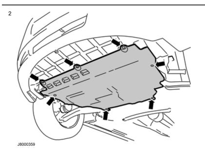
Unscrew the screws and remove the engine splash guard.
