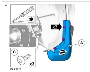
Install and screw the mudflap into place.
