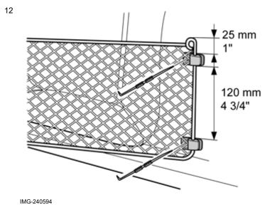
Fit two clips on the net's front end panel in the positions illustrated.
