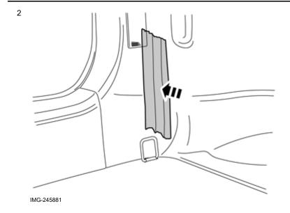
Affix of strip of tape in the rear edge of the cargo compartment's left panel as illustrated.
