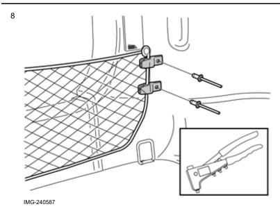
Rivet the rear end panel clips in the side panel.
