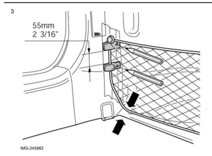
Position the rear end panel of the net against the rear edge of the side panel and position the front end panel against the side of the side panel so that the moveable part of the cargo compartment mat does not catch the rear net end when it is raised.
