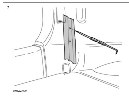
Press a scriber through the markings on the tape strip and through the panel to create holes about  $\varnothing$  4.8 mm (3/16") in diameter.
