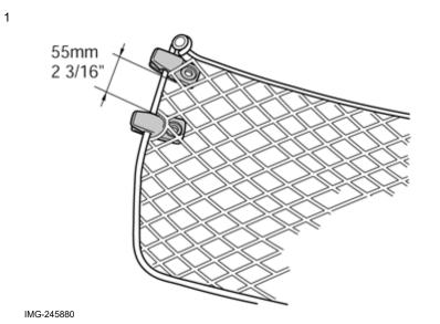
Take the net from the kit and press two of the clips into the rear end panel. The upper clip should be high up on the end panel and the lower as per specified measurements.
