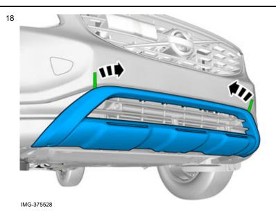
**Hint**Press and apply pressure to the part over the tape for at least 20 seconds.
