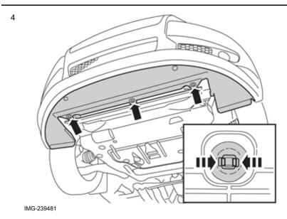
Remove the three plastic clips in the lower edge of the bumper casing.
