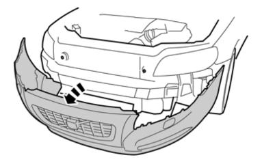
Tilt the bumper casing forward to access the rear of the grille.
