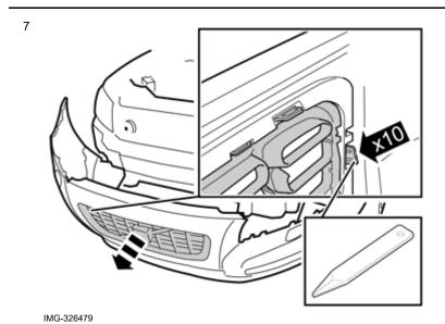
Take a weatherstrip tool and carefully pry up the holes for the grille's catches all the way around so that they can be pushed out and the grille removed. Place to one side. A new grille can be found in the kit.
