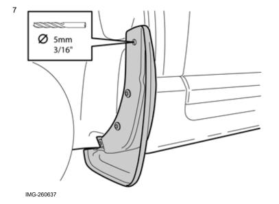
Drill a new 5 mm (3/16) hole at the marking.
