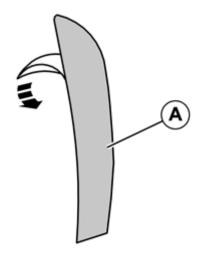
Remove the backing paper from the tape (A).
